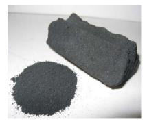
Raw materials – Activated charcoal is a natural material. As such, there is substantial variability between raw material sources, even within a given purchase lot or within an individual shipping container. Diverse sampling and accurate measurement is required to obtain a clear picture of the exact characteristics of the granular carbon and additives to predict how they will interact and perform in the production process. Raw material blending ratios are defined and captured in the Control Plan.
